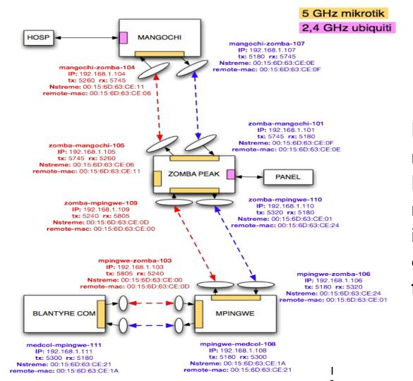
Here is an example of a network plan, with IP and MAC addresses, host names, locations, interconnections, operating bands, and frequency choices.
