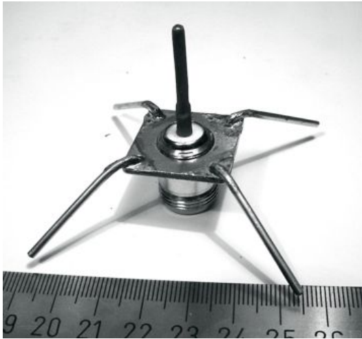
Figure ATL 11: Quarter wavelength ground plane antenna.
