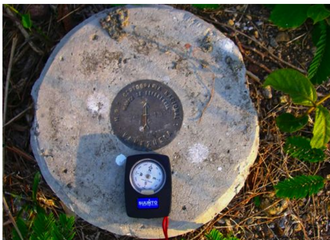
Figure OI 2: Difference between Magnetic and Geographical North at El Baul, Venezuela in 2006.
