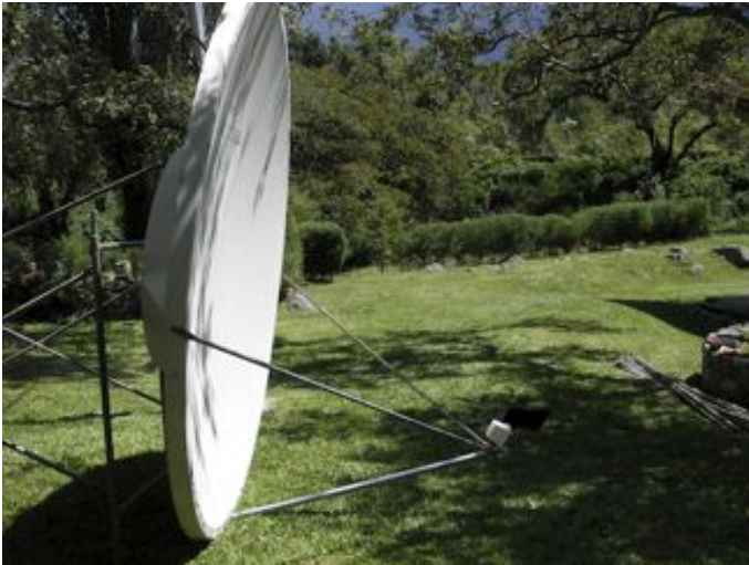
Figure CsLD 4: 2.4 m offset fed reflector with a 12 dBi antenna at its focus, looking 14° down. The actual elevation is 8° up.
