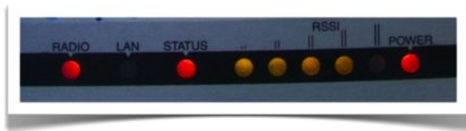
Figure HW 4: The front of a typical Access Point.
