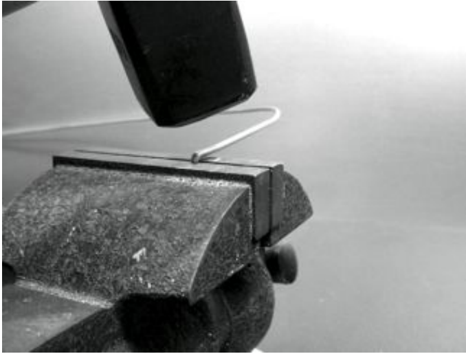
Figure AC 3: Gently tap the wire to make a sharp bend.
