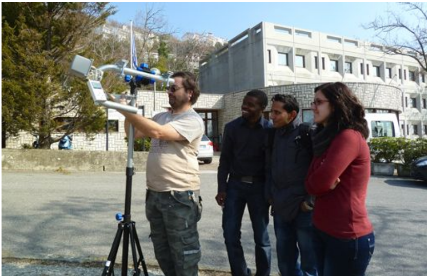
Figure RS 6: Participants from Albania, Nepal, Malawi and Italy testing an antenna with the RF Explorer Spectrum Analyzer in Trieste, February 2012.
