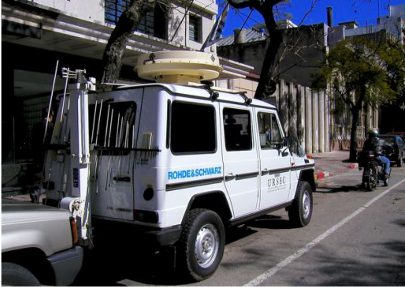
Figure RS 2: A special vehicle for spectrum monitoring in Montevideo, Uruguay.
