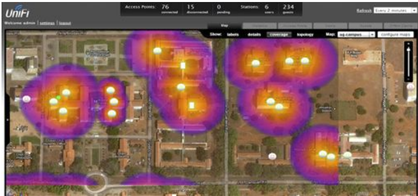
Figure CSG 7: With UniFi we are able to simulate the coverage of the wireless signal as shown above.
