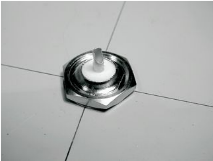
Figure AC 12: Secure the N connector tightly to the plate.
