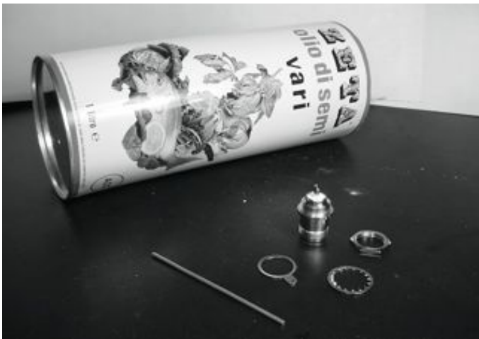
Figure AC 21: Parts needed for the cantenna.
