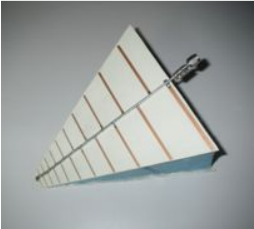
Figure ATL 16: Log periodic antenna
