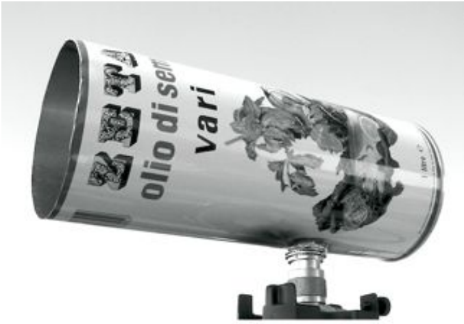
Figure AC 20: The finished cantenna.
