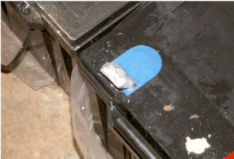
Figure OGP 2: A 200 Ah lead-acid battery. The negative terminal was broken due to weight on the terminals during transportation.
