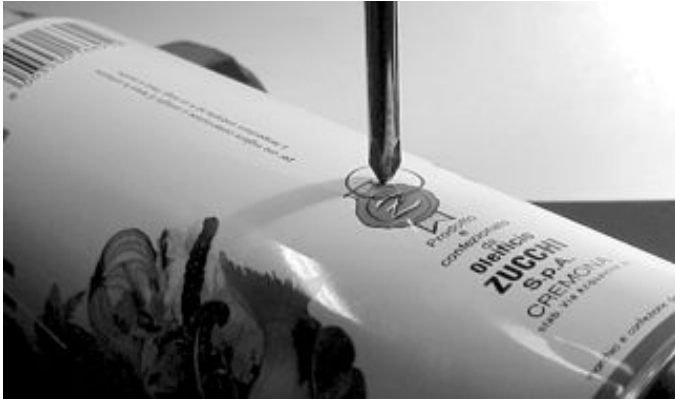
Figure AC 23: Mark the hole before drilling.
