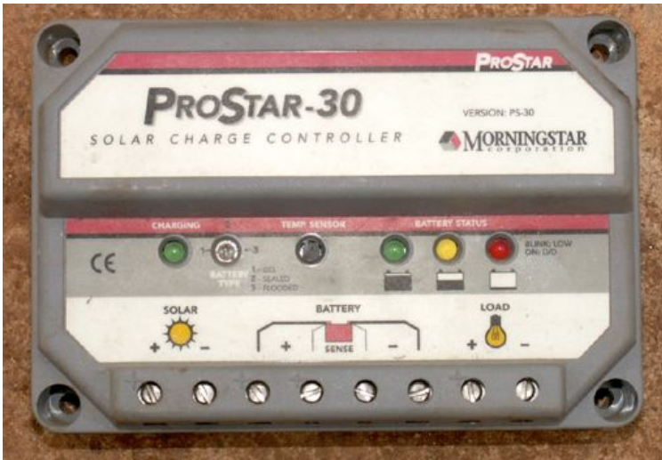
Figure OGP 3: A 30 Amp solar charge controller
