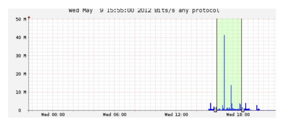
Go to Profile, select the group you created then select 'HTTP\_TRAFFIC'. Then go to the 'Details' tab and select 'Time Window' instead of 'Time Slot' beneath the graph. Choose a part of the graph with activity as above
