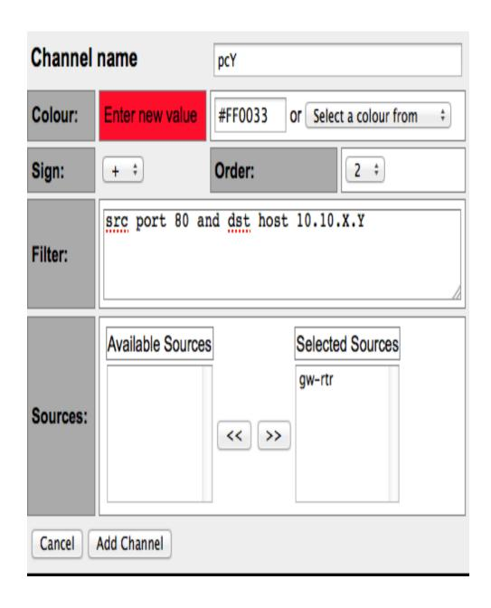
Add another channel by clicking the plus sign as before next to 'Channel List'. Fill the details as shown on the left. Replace Y with the pc number that is **NOT** receiving flows in your pair!
