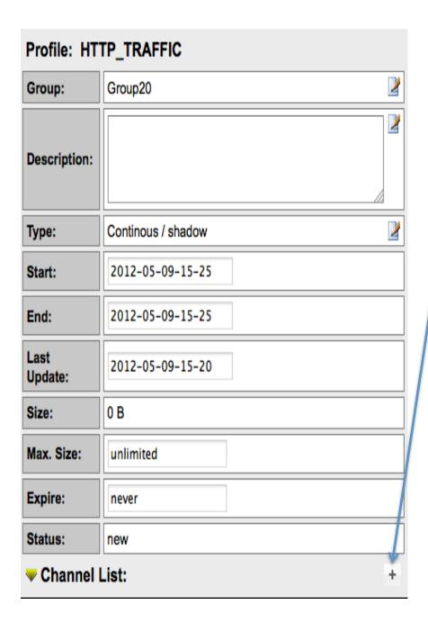
Click on the plus sign next to 'Channel List' at the bottom of the page then fill the next page as below and click on 'Add Channel' at the bottom. The filter 'any' means ALL traffic
