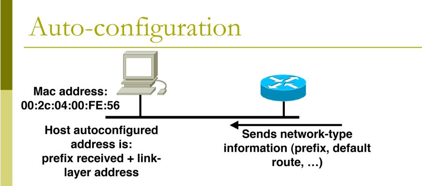
Client sends router solicitation (RS) messages Router responds with router advertisement (RA) This includes prefix and default route Client configures its IPv6 address by concatenating prefix received with its EUI-64 address
