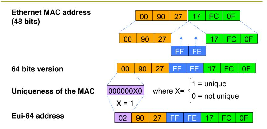
EUI-64 address is formed by inserting FFFE and OR'ing a bit identifying the uniqueness of the MAC address
