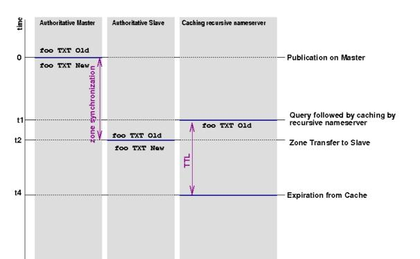
Figure 10: DNS Data Propagation
