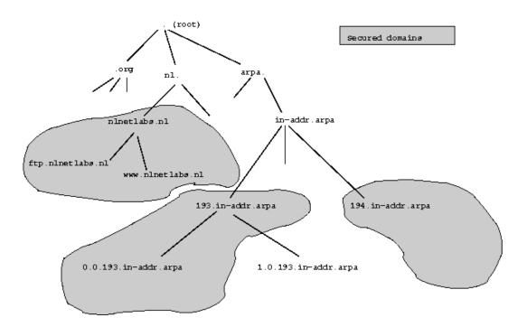
Figure 2: Trust anchors in the DNS tree
